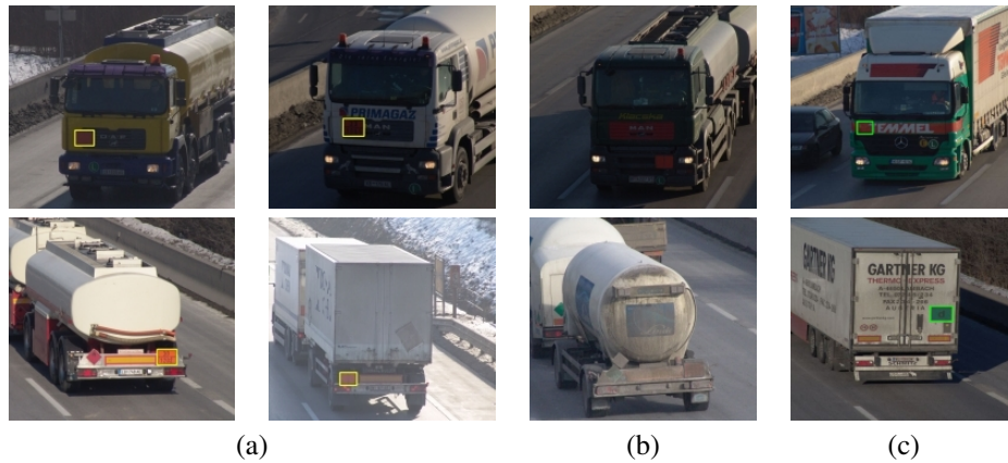
Figure 6: Illustrative detection results - Trucks data set: (a) correctly detected plates, (b) missed plates, and (c) false positives.
