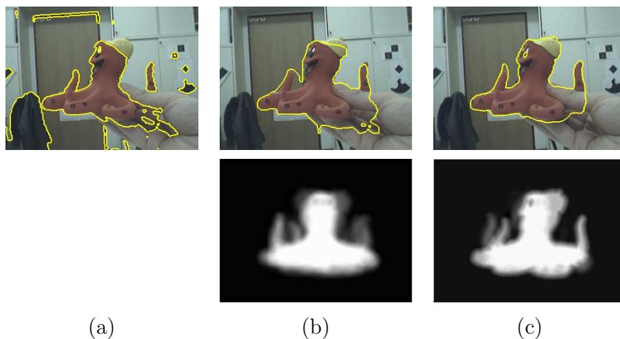
**Figure 4: Estimated shape prior and corresponding level set segmentation: (a) without an ASM, (b) with an ASM learned from 40 training shapes and (c) with an ASM learned from 80 training shapes.**
