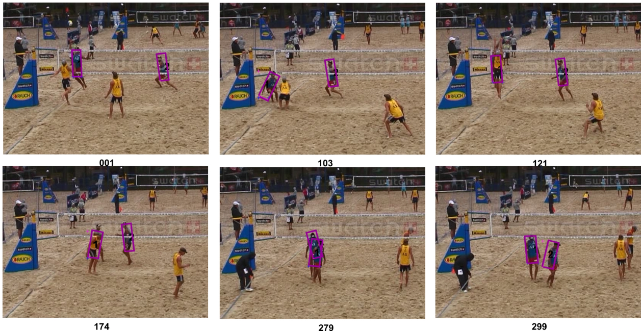
Figure 5: Tracking results of the final method. During occlusions from opponent players, the tracker follows the occluding player, frames 121 and 174. After an intersection in frame 279 particle sets are separated again but identities are switched.
