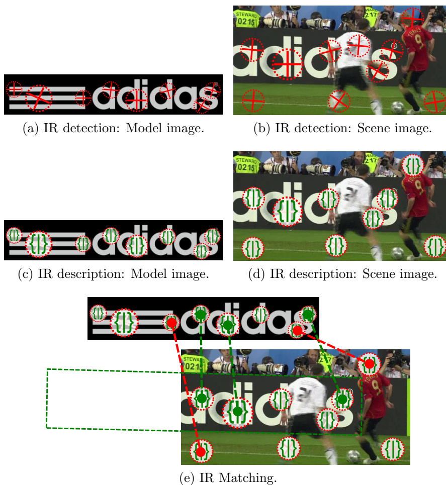
Figure 2: Basic flow of object recognition with local features: Interest regions (IRs) are extracted (a)-(b) and described (c)-(d). Interest region correspondences are formed (e). The green lines indicate correct match correspondences, estimated pose shown in dashed green.
