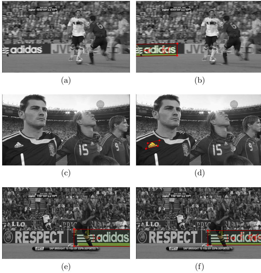
Figure 10: Model family approach (right column) compared to standard approach (left column). The red arrows indicate pose consistent succeeding matches.
