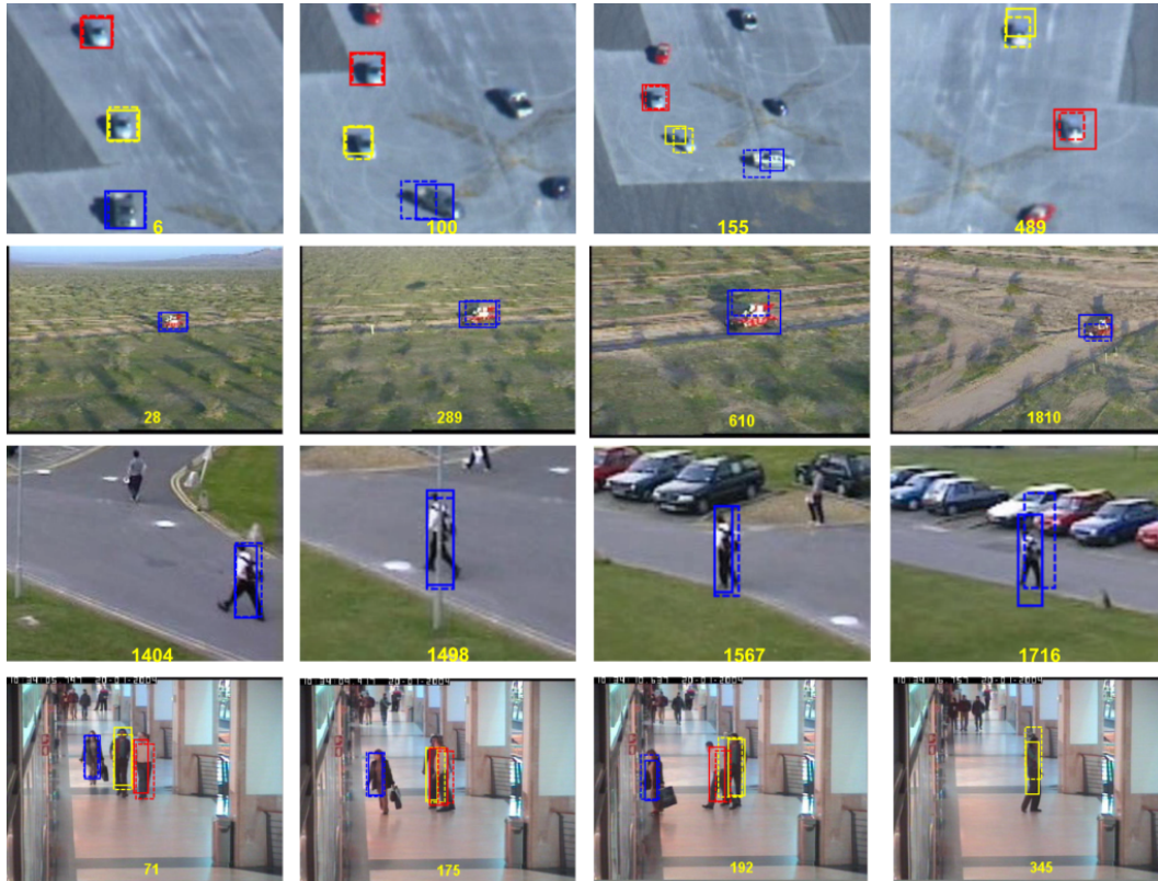
Figure 5: Improvements to the proposed sub-parts tracker (dashed), using the incremental eigenspace representations for each sub-part (solid).
