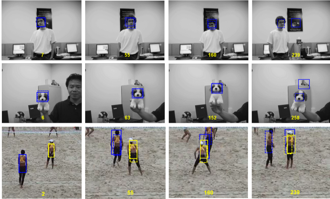
Figure 4: Visual tracking results of the covariance descriptor proposed in [17] (solid) compared to our part based tracker using Euclidean approximation of covariance matrices (dashed).
