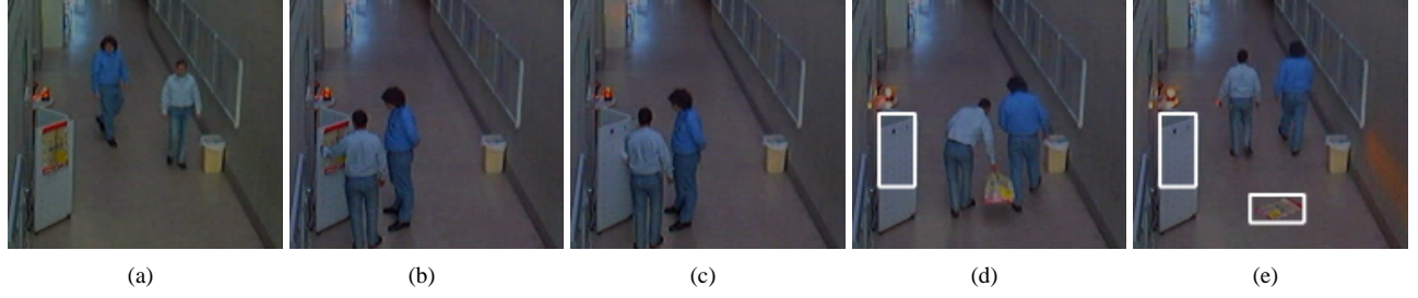
Figure 6: CoffeeCam / Larceny Scenario - Changes in the background model: (d) the missing poster (object removed) and (e) the poster lying on the floor (object added) are detected.
