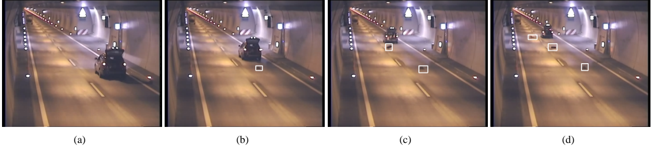
Figure 7: Tunnel Safety - Objects that were thrown out of the car are detected: (a) no object, (b) chock, (c) car tire, (d) safety cone.
