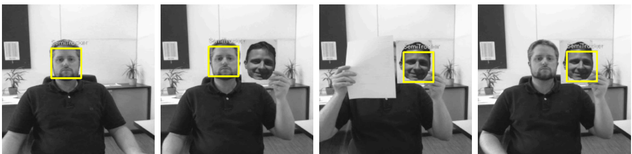
(a) Tracking a face, using a class-prior (b) Two faces within search space (c) Classifier switches to other face and starts adapting (d) Finally tracking the other face
