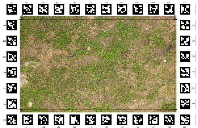
Figure 5: Target with fiducial markers to be tracked by ARToolkitPlus and content tracked by NaturalFeatureTracker.
