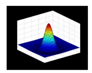
$$DOG(x,y) = \frac{1}{k}e^{-\frac{x^2+y^2}{(k\sigma)^2}} - e^{-\frac{x^2+y^2}{\sigma^2}}$$
