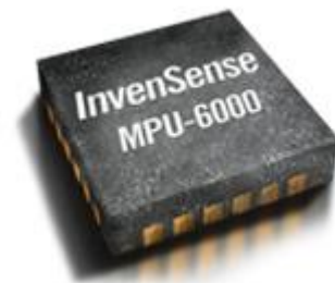
Invensense MPU-6000, 0.1 g, MEMS, 4x4x0.9mm
