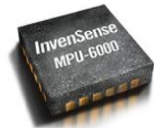
Invensense MPU-6000, 0.1 g, MEMS, 4x4x0.9mm
