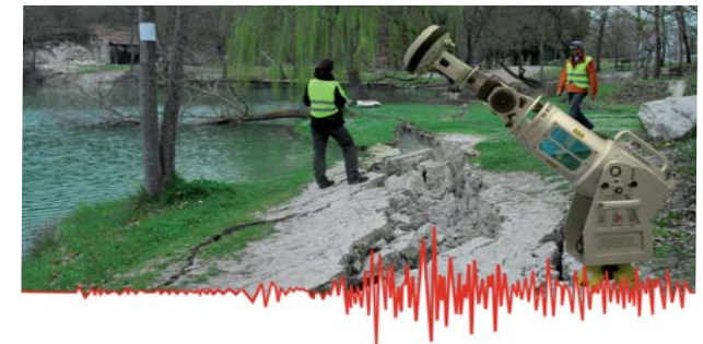
LiDAR survey of ground failure caused by the 2009 L'Aquila Italy earthquake
