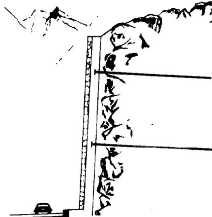
Figure A-13 – Rock face revetment, Switzerland
