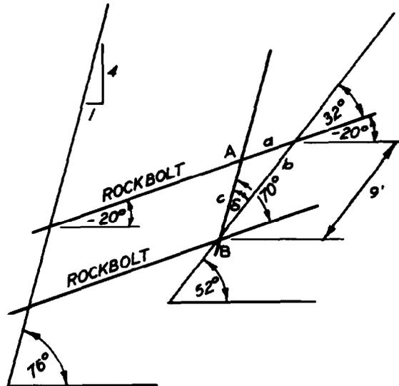
Figure 3-16. Calculation of actual bolt spacing for FS = 1.1.
