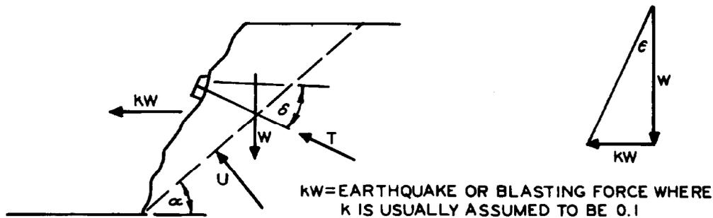
Figure 3-15. Force polygon for earthquake or blasting force.
