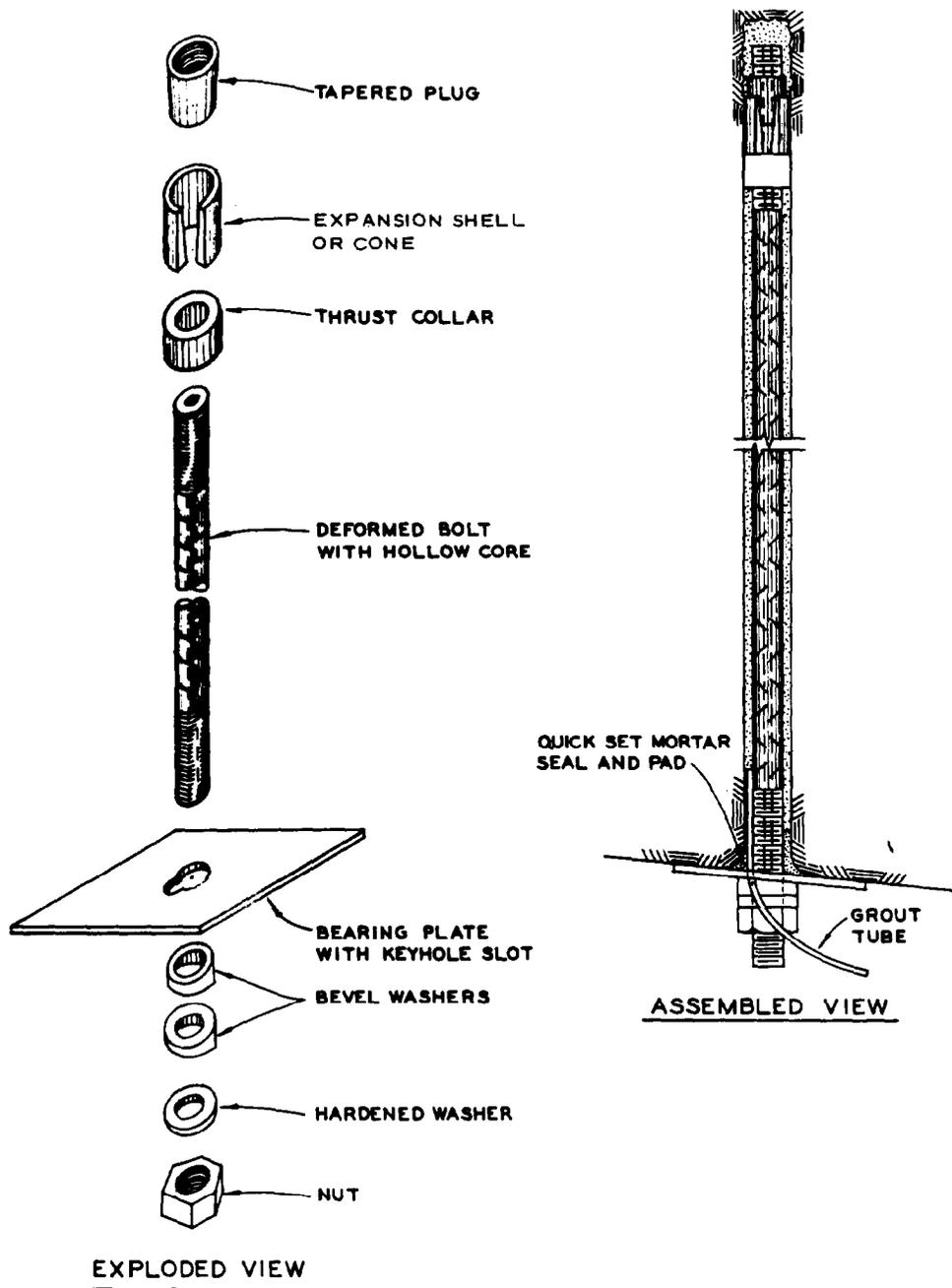
Figure 3-5. Hollow groutable deformed bar rock bolt.
