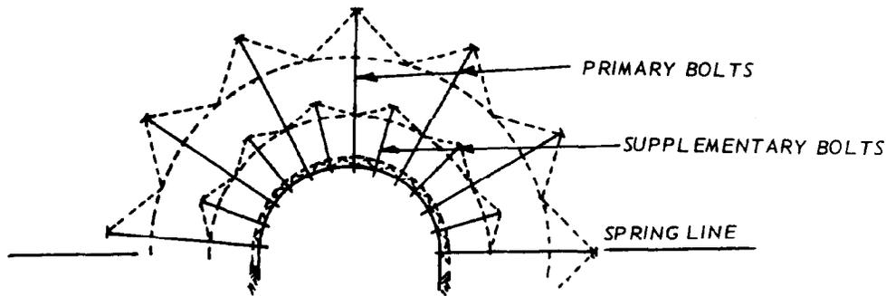
Figure 2-9. Supplementary rock reinforcement.
