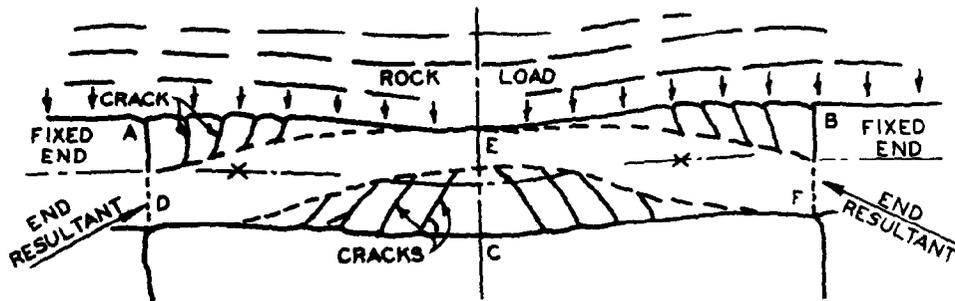
Figure 2-4. Mode of failure of uniform material beam.
