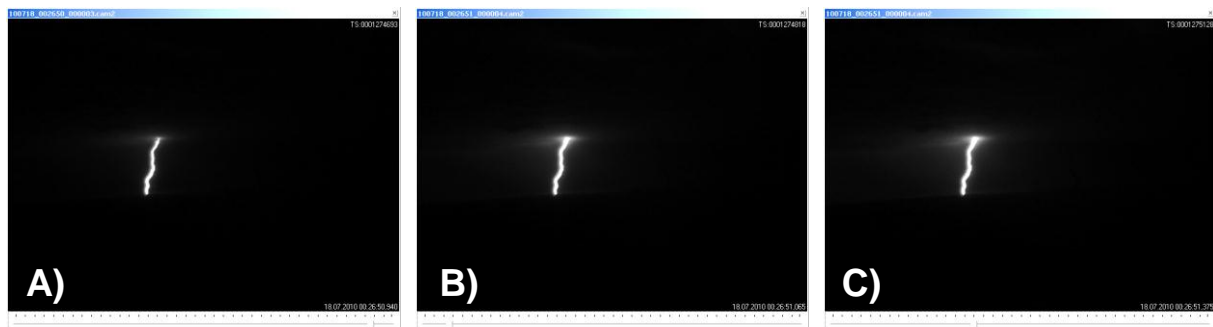
Figure 6: A), B) and C) show three strokes out of a four stroke flash. All these strokes follow the same channel to ground and were detected by ALDIS. Therefore ALDIS provided location data for each of these flashes and distances between location of A) and B) as well as A) and C) can be calculated. Note: This Figure shows images out of the continuing current sequence because the images of the return stroke sequence are saturated.
