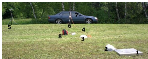
Figure 2: VFRS deployed in the field. 1-flat plate antenna, 2-integrator amplifier, 3-fibre optic transmitter, 4-fibre optic cable, 5-high speed camera, 6-GPS antenna, 7-VFRS components inside the car, 8-power supply. Note: The generator is typically 50 m distant from the car and the antenna deployed.
