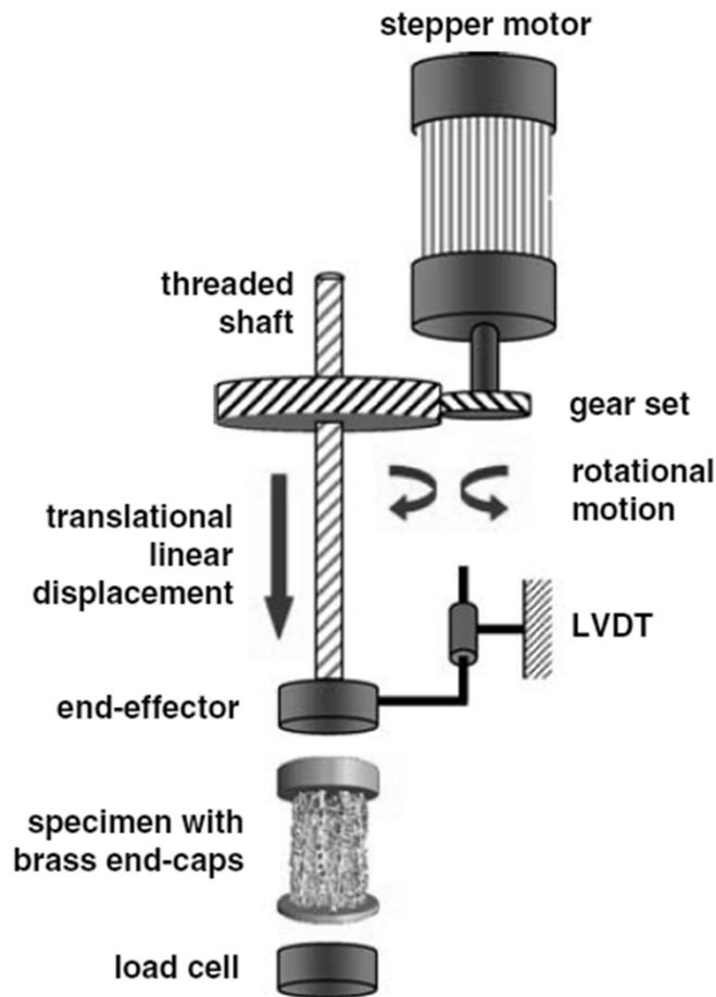
Linear variable Differential-Transformators (LVDT)
