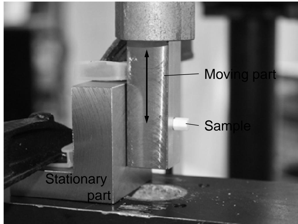
Bone screw in the testing apparatus
