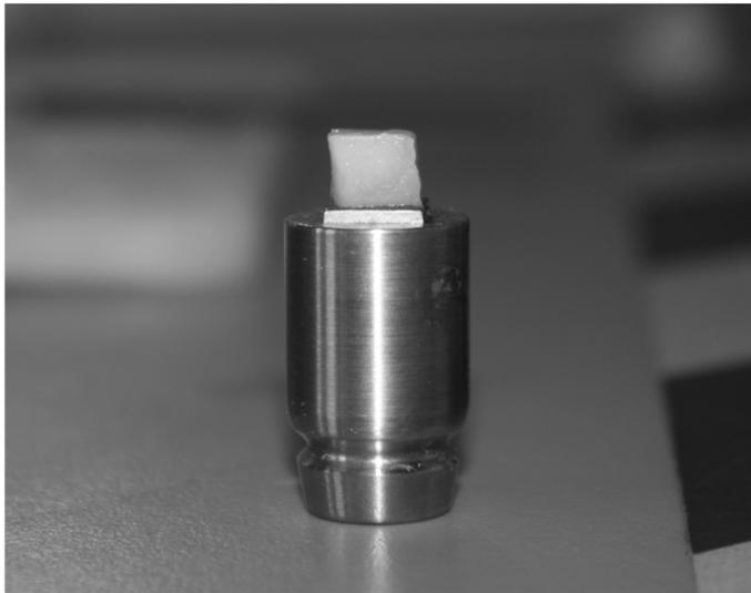
Specimen glued to specimen-holder
