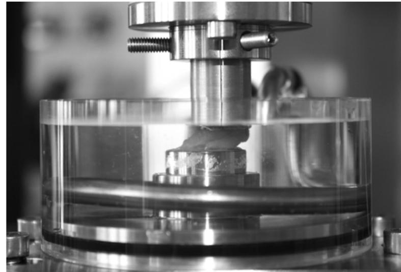
Specimen during shearing
