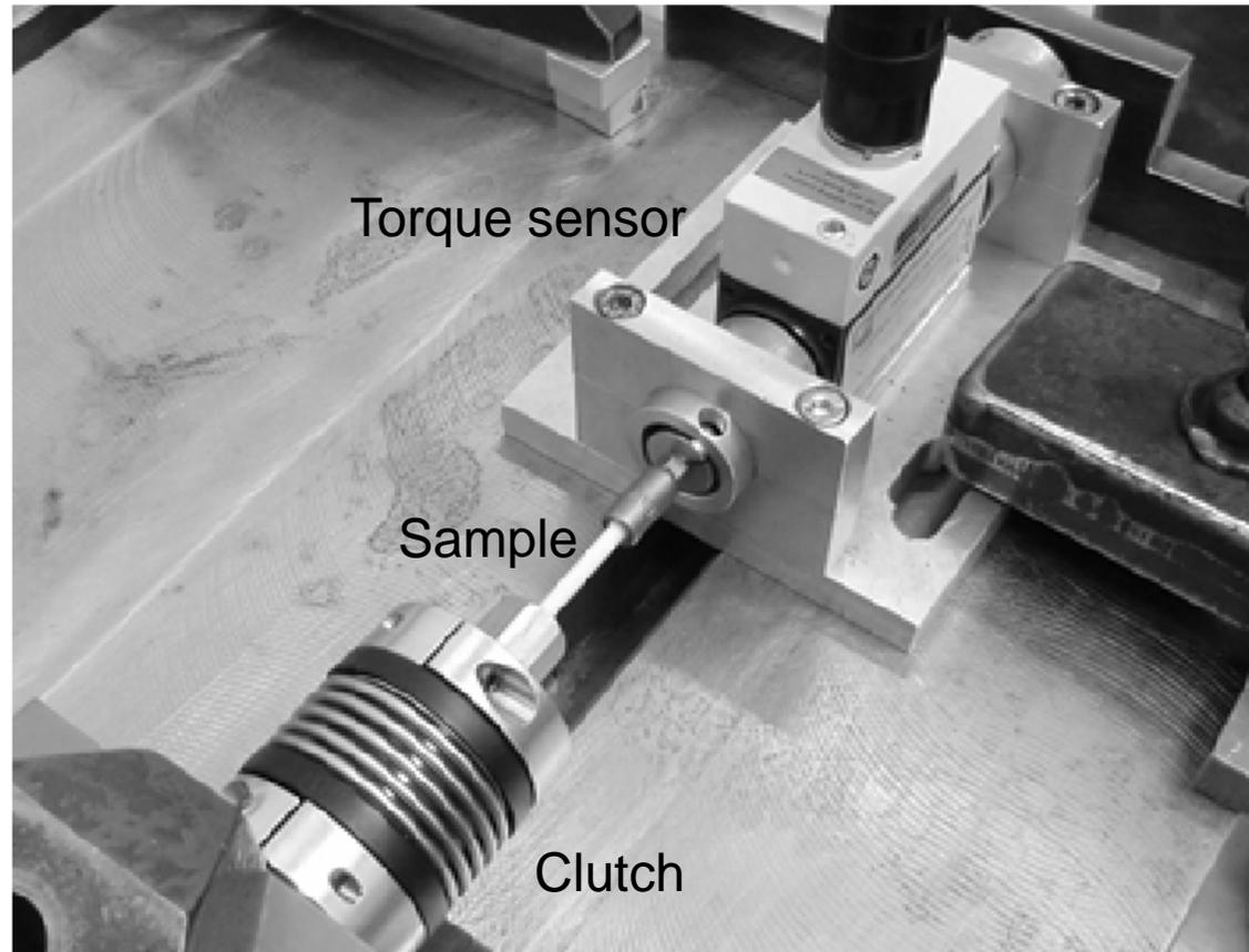
Bone screw in the testing apparatus
