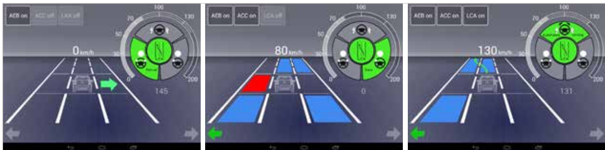
Figure 1: HMI for different automation levels: a) manual, b) semi-automated and c) automated
