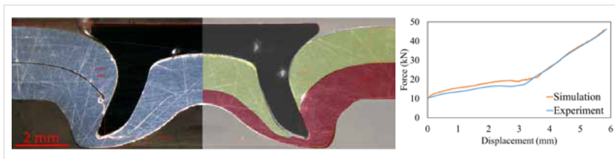
Figure: Comparison between experiment and simulation: SPR joint cross-section (left) and punch force-displacement curves (right)
