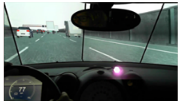
Fig. 2: Experiment of a volunteer driver in a dense traffic on a highway. The driving simulator is an open platform to integrated automated driving and test the human-machine interaction in a reproducible way.
