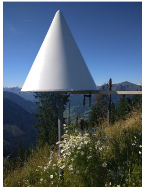
Figure 2. Corner reflector: to monitor ground motions precisely in areas where no other artificial or natural reflectors are available. © GEORESEARCH Forschungsgesellschaft mbH
