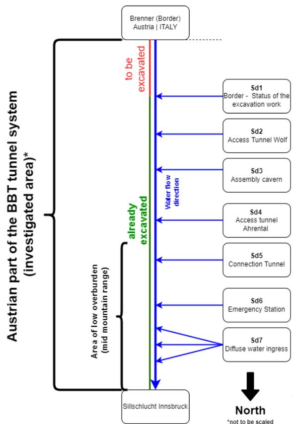
Figure 1. Tunnel water discharge system at the Austrian section of the BBT. [4]
