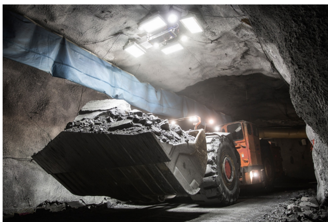
Figure 1: Setup for data acquisition in LKAB's Kiruna mine for the determination of the fragment sizes in a muck pile (c) LKAB, Runar Gudmundsson.
