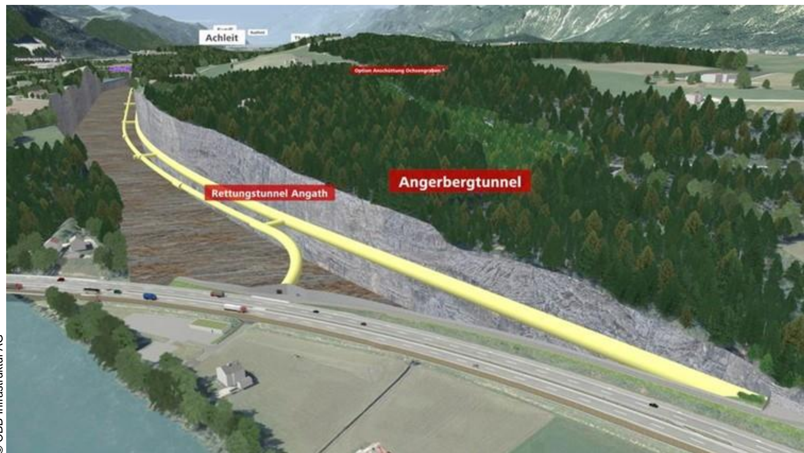
Alignment of the Angerberg tunnel with the accompanying Angath rescue tunnel.
