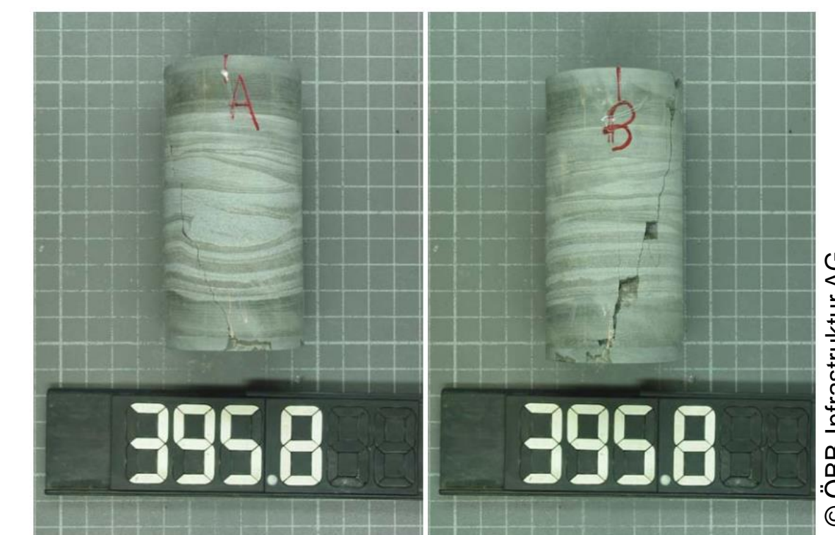
Sample before and after a uniaxial compression test in directions A and B.
