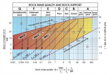
Permanent support recommendations based on Q-values and span/ESR
