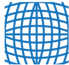
Positive radial distortion "barrel"
