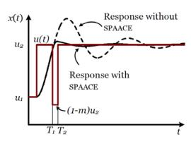
monitoring the response and temporarily modulating the set point. The salient features of this strategy are (i) robustness with respect to system parameters, (ii) independence of system model, (iii) reliance merely on local signals, and (iv) absence of need to adjust existing controllers. The proposed control strategy and its performance are discussed and evaluated, and its technical feasibility is established through a number of case studies.
