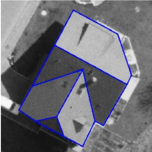
Figure 6: Result of automatic roof reconstruction (source: [16]).
