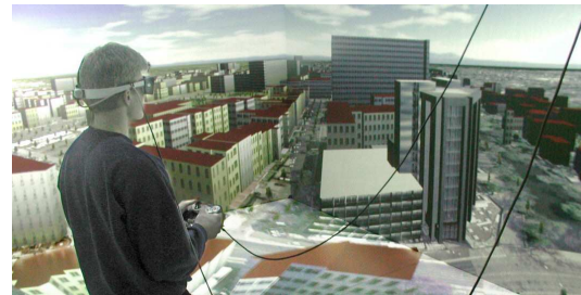
Figure 11: Exploration of the 3D city model of Braunschweig in a CAVE. A manually modeled landmark is visible.
