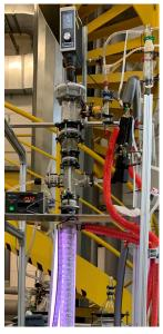
The Taylor-Couette Disc Contactor (TCDC) is a novel extraction device developed at the institute that can be used for a variety of separation tasks comprising various phases. To improve comparability with conventional devices and scale-up, several bachelor theses / plant design exercises are scheduled to systematically investigate the TCDC's power consumption.
