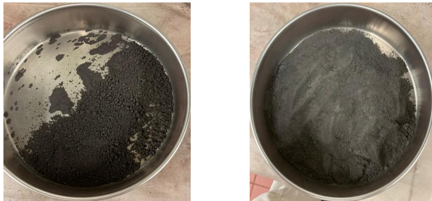
Fig. 1: Oxygen carriers with particle size 180-250 \mu\text{m} , synthesized from pure manganese oxide powder (left) and synthesized from manganese ore (right).
