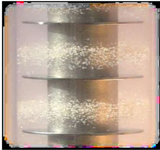
Figure 1: Solid sodium chloride particles which are held in levitation by Taylor-Couette vortices
