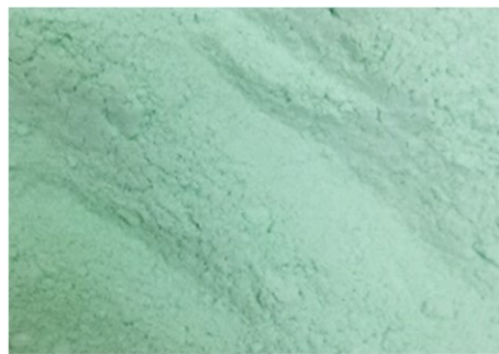
Fig. 2: Ni/MgO catalyst after impregnation
