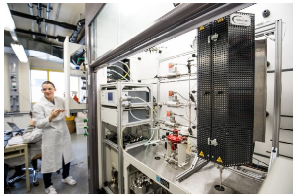
Fig. 3: Setup of the tubular reactor from parr industries The feed gas ratio was H 2 :N 2 :CO 2 =56:30:14. Feed gas streams from 1.2–14.8 m 3 kg -1 h -1 and temperatures between 260°C and 425°C were tested.
