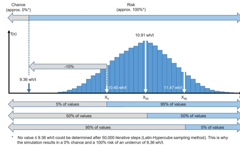
Figure 2: Distribution as a result of a Monte Carlo simulation to illustrate how to determine a labor consumption rate minimum for reinforcing works
