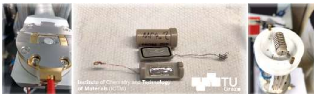
Figure 1: Typical lithium-ion battery active materials react with components of the ambient atmosphere and must therefore be handled under inert-gas conditions. Specialized sample holders are required to enable electrochemical reactions while remaining compatible with in-situ measurements. A coin cell sealed with a 20 \mu\text{m} thin Al current collector that also serves as an X-ray transparent window for monitoring phase changes during reaction progress (left). A metal-free cell housing designed for NMR measurements and fitting into the coil of a dedicated NMR probe is shown in the middle and right panels.
