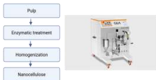
Figure 1. Process scheme and homogenization equipment
