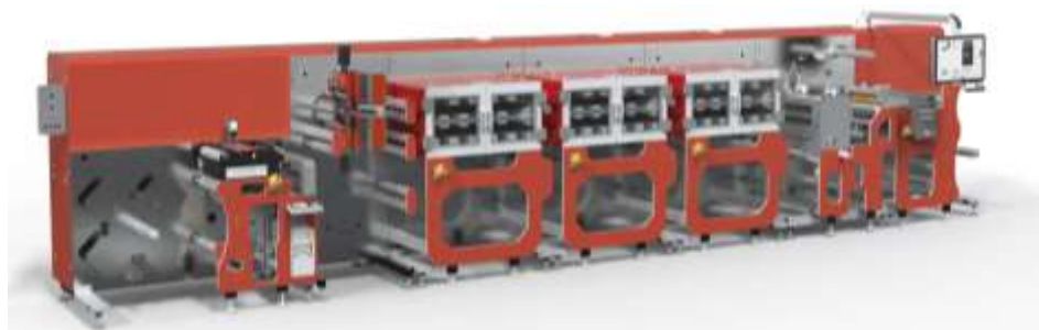
Figure 1: Roll-to-Roll Coater (Sample image: FOM moduloR2R)
