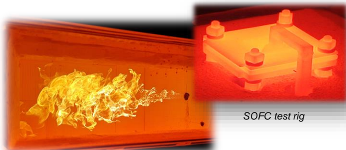
Flame in a 1.5 MW burner chamber with optical measurement system
