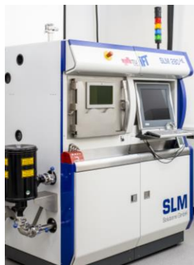
Selective laser melting system (AddLab @tugraz)
