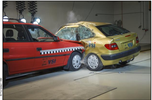
Full-scale crash test as part of a laboratory exercise
