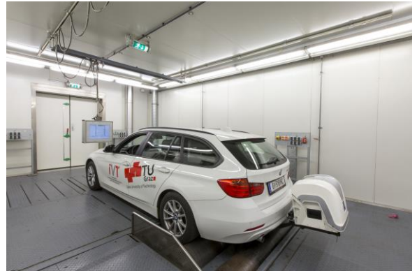
Emission measurements on the chassis dynamometer with OnBoard measurement equipment
