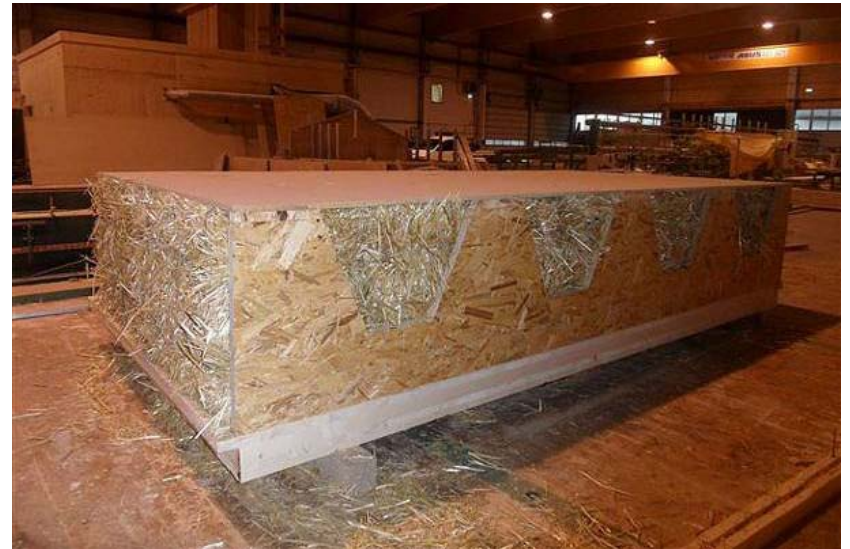
prototype element with cover panel, pressed in vacuo
