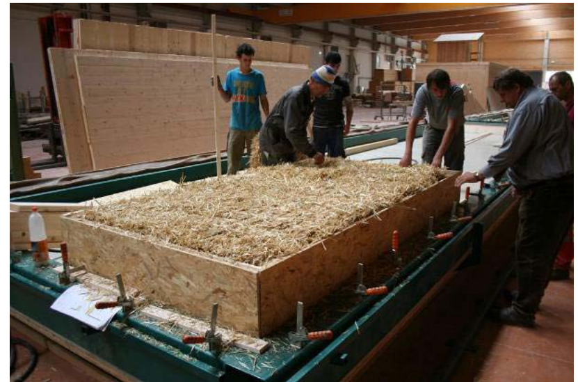
inserting straw bales
