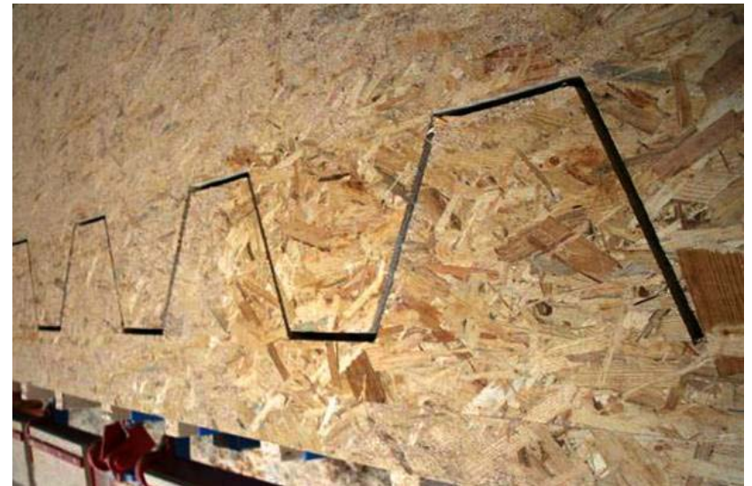
cutting of components: composite lumber and OSB
