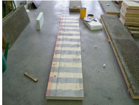
Composite beam: glass fibre mat with two-component adhesive
