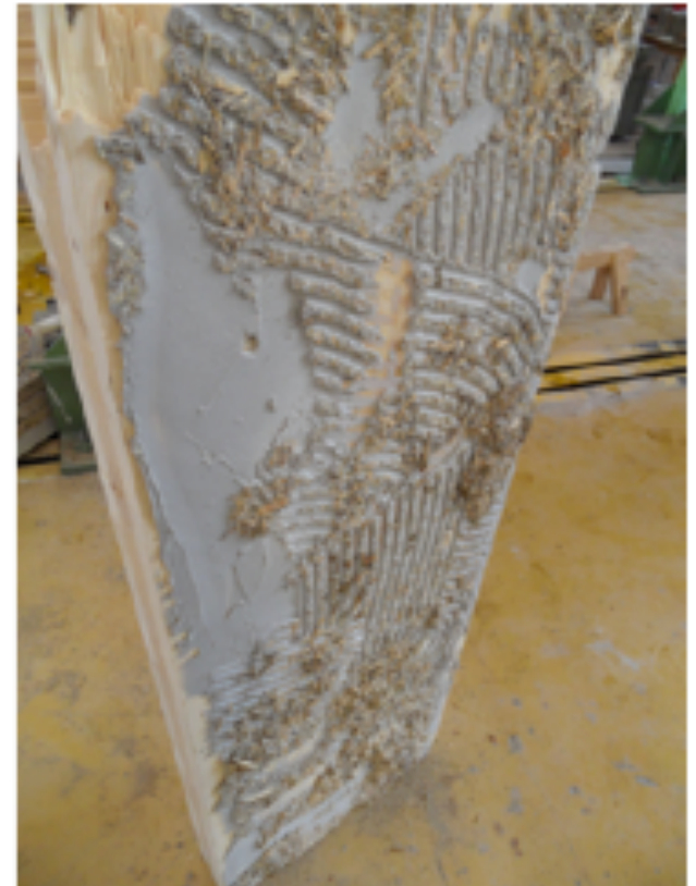
Composite beam: glass fibre mat with two-component adhesive
