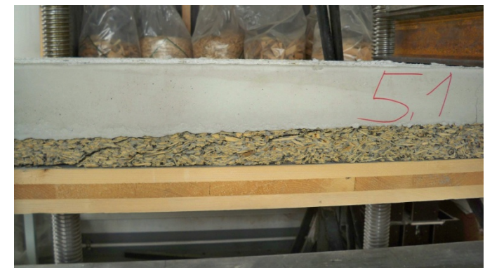
Test Nr. 5: two-component adhesive
