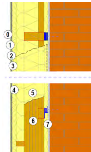
Wood construction. Prefabricated including insulation material, plastered
