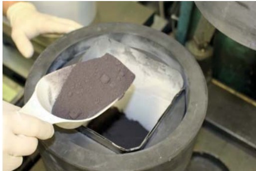
Figure 7: manually filling of Si powder into the graphite pressing mold
