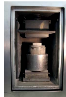
Figure 10: hot pressing machine with completed pressing mold
