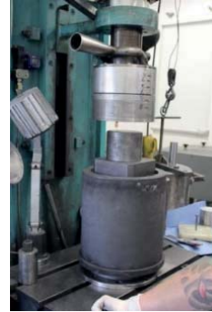
Figure 8: cold pre pressing of Si powder in the completed pressing mold
