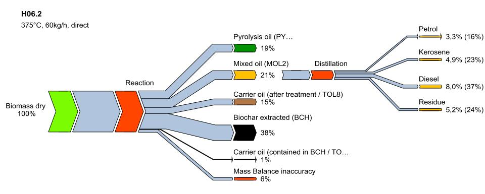
Results from bioCRACK pilot plant Schwechat Feedstock: spruce
