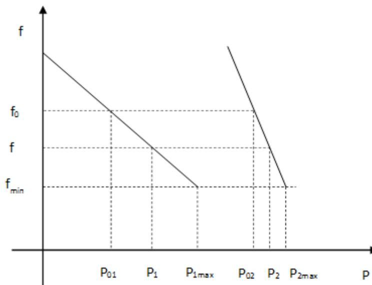
Figure 1. Active power / frequency droop control characteristic [3]
