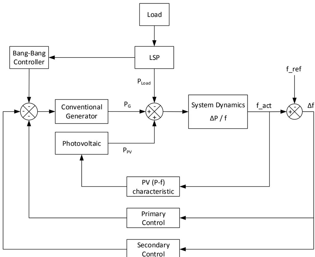
Figure 3. Schematic block diagram of islanded microgrid
