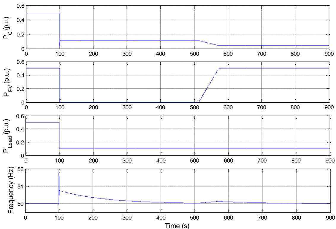
Figure 7. Dynamic simulation results ( $P_G$ : the power output of the conventional generator;  $P_{PV}$ : the power output of the PV;  $P_{load}$ : the power consumption of the load; Frequency: the system frequency)
