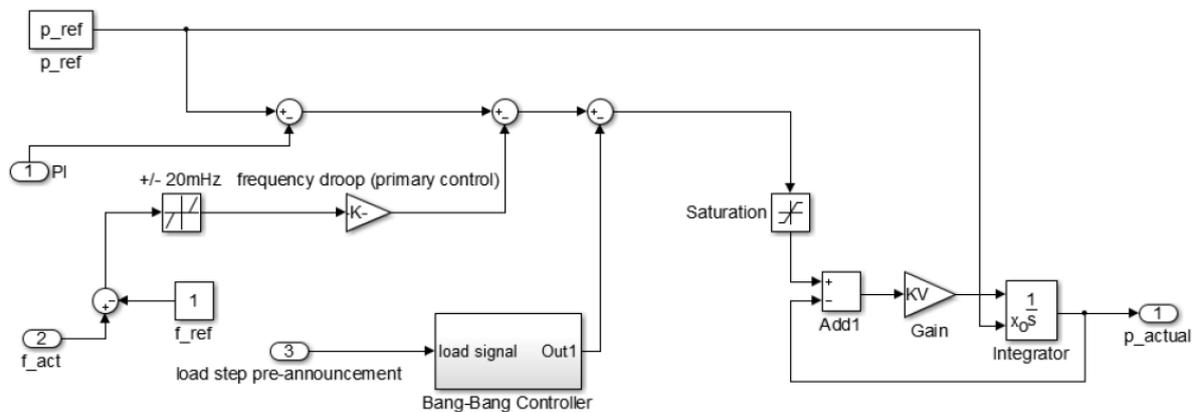
Figure 4. Conventional generator simulation model
