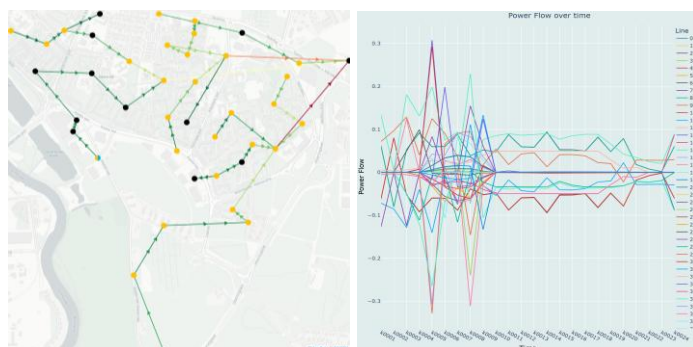
Figure 1: Grid utilization and renewable production at a given time t (left) and active power-flow of each line over the modeling horizon (right).
