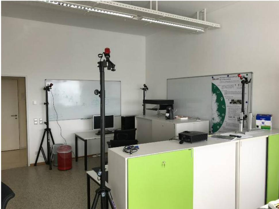
**Abb. 4.1.2:** Spatial Tracking Setup in the Lab
