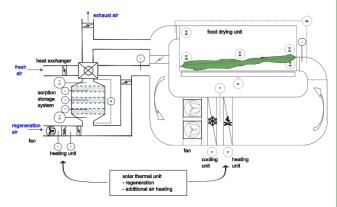
mobile drying system consists of an optimized combination of a sorption storage system, a solar thermal collector and heat recovery. The aim of this Master's thesis is to develop and validate a superordinate operating strategy for a prototype (see figure) to achieve high product quality through precise control of the drying good's moisture, and an intelligent combination of the individual components of the drying system to increase efficiency.
